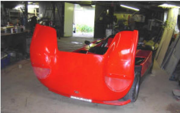
The nose and rear pivot forward and backward respectfully and the scuttle panel can be removed with 8 quick release screws leaving a bare chassis, suspension and engine transaxle fully open to work on!
